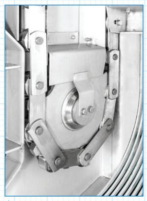
A Option 2 Heavy-duty stainless steel chain and lower sprocket engagement system
