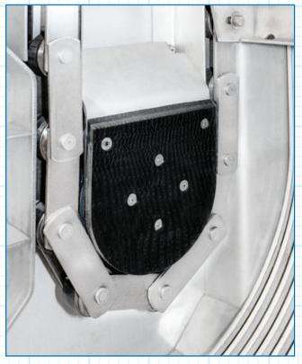
A Option 1 Heavy-duty stainless steel chain and lower guide rail engagement system
