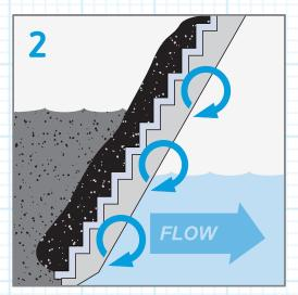
When the differential or high level reaches a predetermined level, the movable lamellas are activated. The movable lamellas rotate upward, lifting the debris to the next highest level of fixed lamellas, and then rotate back to their original position. The drive system provides a positive mechnical action throughout the complete rotation of the movable lamellas. This enables the unit to drive through any debris that may accumulate under the screening surface.
